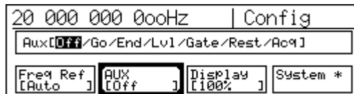
Figure 4.3.15-6 AUX Signal Selection Screen
