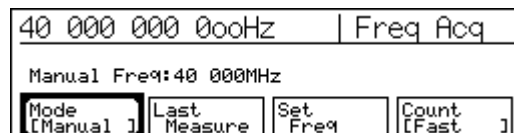
Figure 4.4.2-1 Frequency Acquisition Setup Screen
