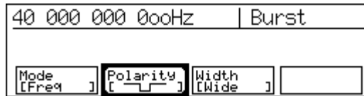
Figure 4.4.7-3 Burst Measurement Polarity Selection Screen
