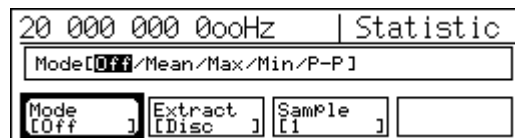
Figure 4.3.11-2 Statistical Processing Mode Selection Screen
