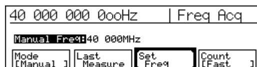
Figure 4.4.2-2 Manual Frequency Value Input Screen
