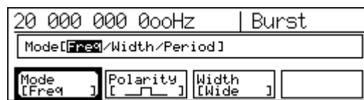
Figure 4.3.7-2 Burst Mode Selection Screen
