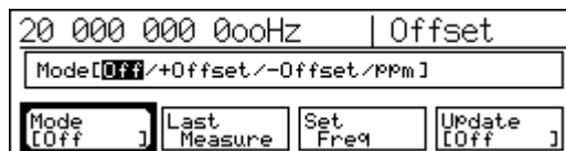
Figure 4.3.10-2 Offset Mode Selection Screen
