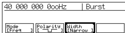
Figure 4.4.7-4 Burst Width Selection Screen
